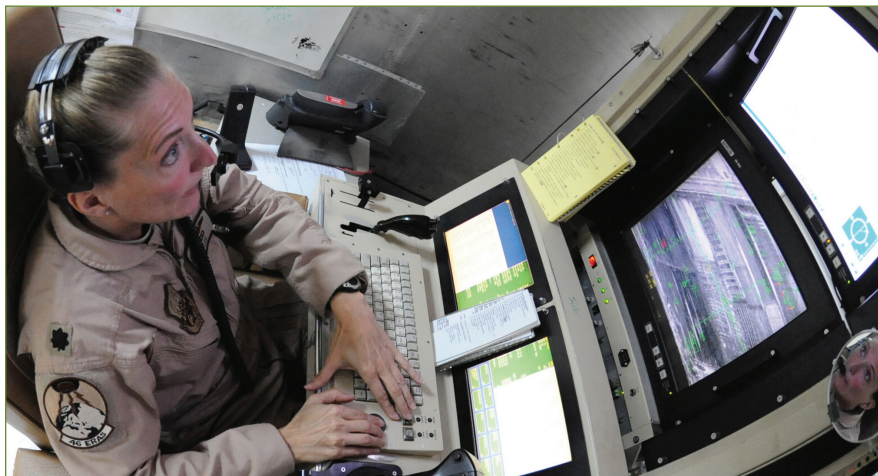
Figure 1 | Practically speaking, without FMV from the aircraft's onboard cameras, pilots would not be able to navigate the UAS remotely from the ground. U.S. Air Force photo by Senior Airman Tiffany Trojca
