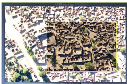
Figure 2 | Many different types of algorithms are important for UAS applications. On this display, an algorithm dehazes images for fog, smoke, and sand-storm environments.
